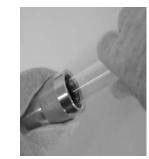
7. Gently slide the dome "O" ring (4032) over the top (open end) of the quartz dome to about 1" from the open end.
